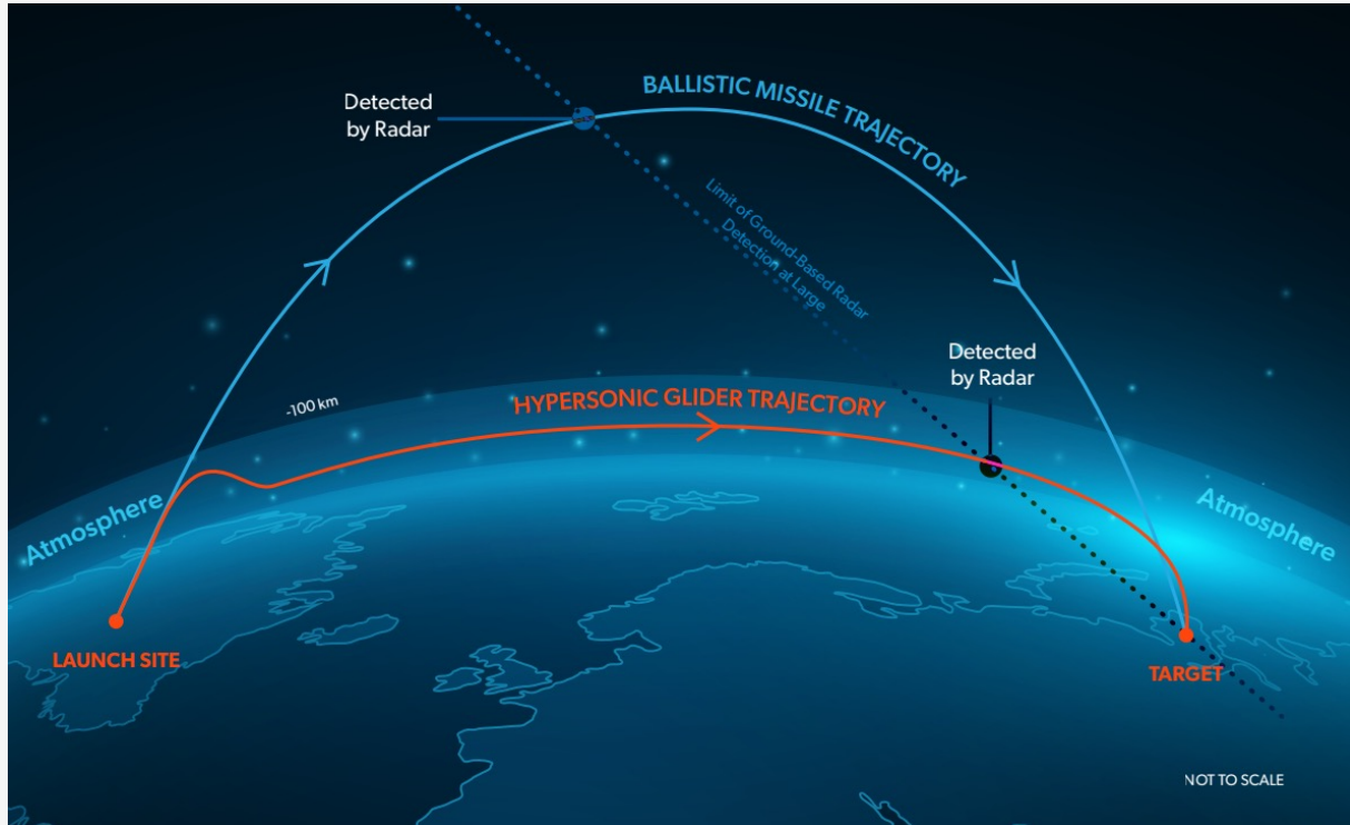
Figure 1: Graphic of radar blind zones in detecting and tracking ballistic missiles and hypersonic glide vehicles trajectories.
